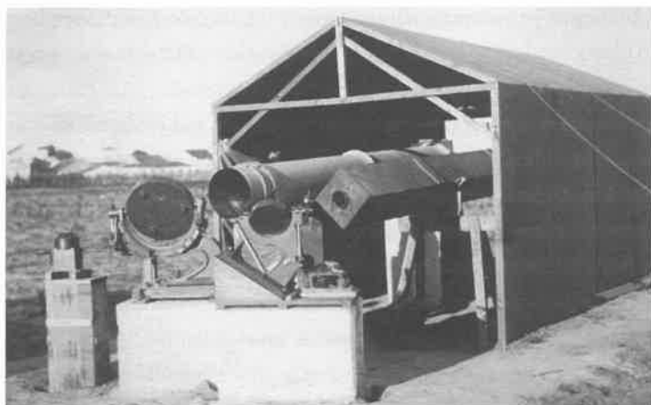
Figure 3.2. The setup of the Eddington expedition's telescopes in Brazil. The astrographic is on the left, the 4-inch on the right. The external mirrors are mounted on the block in the foreground.
